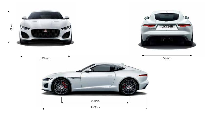
Dimensions were measured with vehicle at unladen weight. ^ DRY: volume as measured with VDA-compliant solid blocks (200mm x 50mm x 100mm). ^^ WET: Volume as measured by simulating the loadspace filled with liquid.
